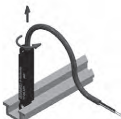
4. Turn the transmitter 90° anti-clockwise and lift out.
