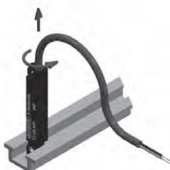
4. Turn the transmitter 90° anti-clockwise and lift out.
