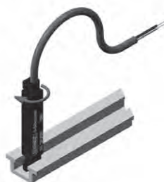
2. Turn the transmitter 90° clockwise.
